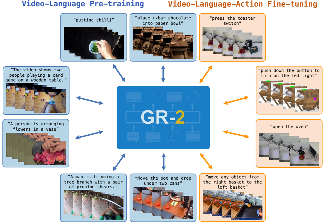
Figure 1: Overview. GR-2 undergoes two stages of training: video generation pre-training and robot data fine-tuning.
