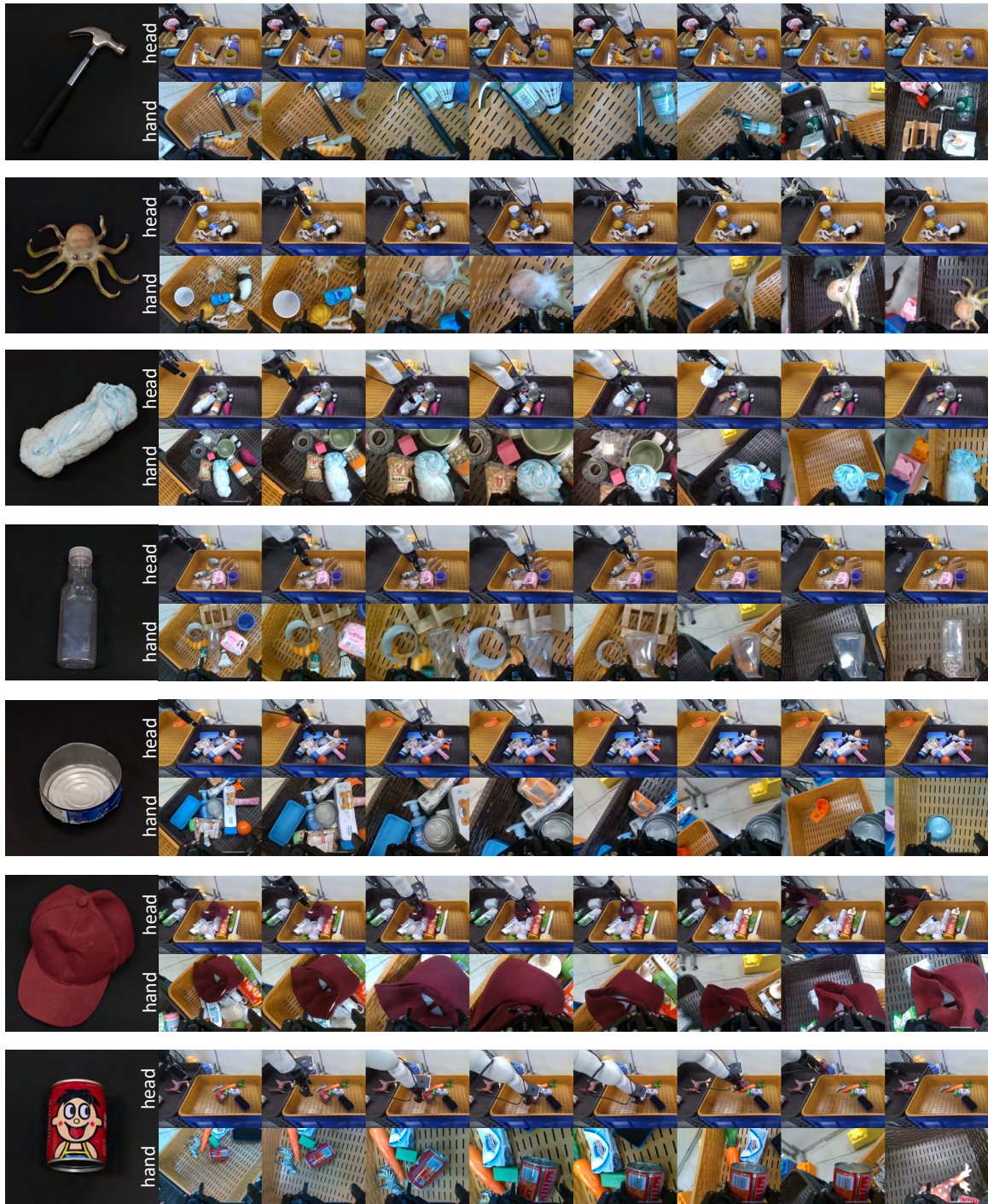
Figure 8: Qualitative Results of End-to-End Bin Picking. We show end-to-end picking of different objects, including objects that are transparent, deformable, or reflective.
