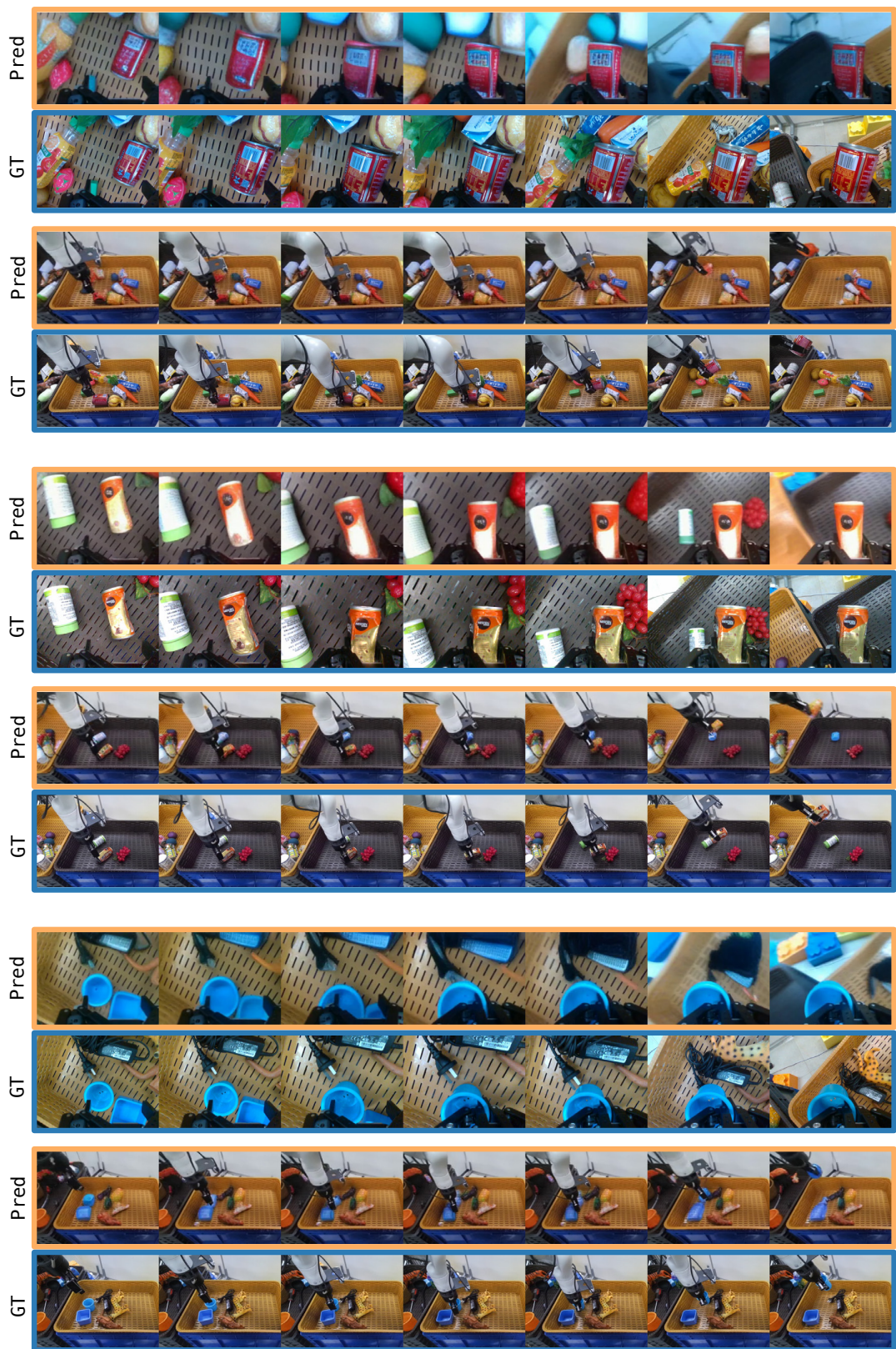
Figure 14: Video Prediction (Pred) and Ground-Truth (GT) Rollouts of End-to-End Bin Picking (I). We show autoregressive video predictions alongside the corresponding ground-truth videos captured from real-world rollouts. Both the views from the hand camera and the static head camera are shown.
