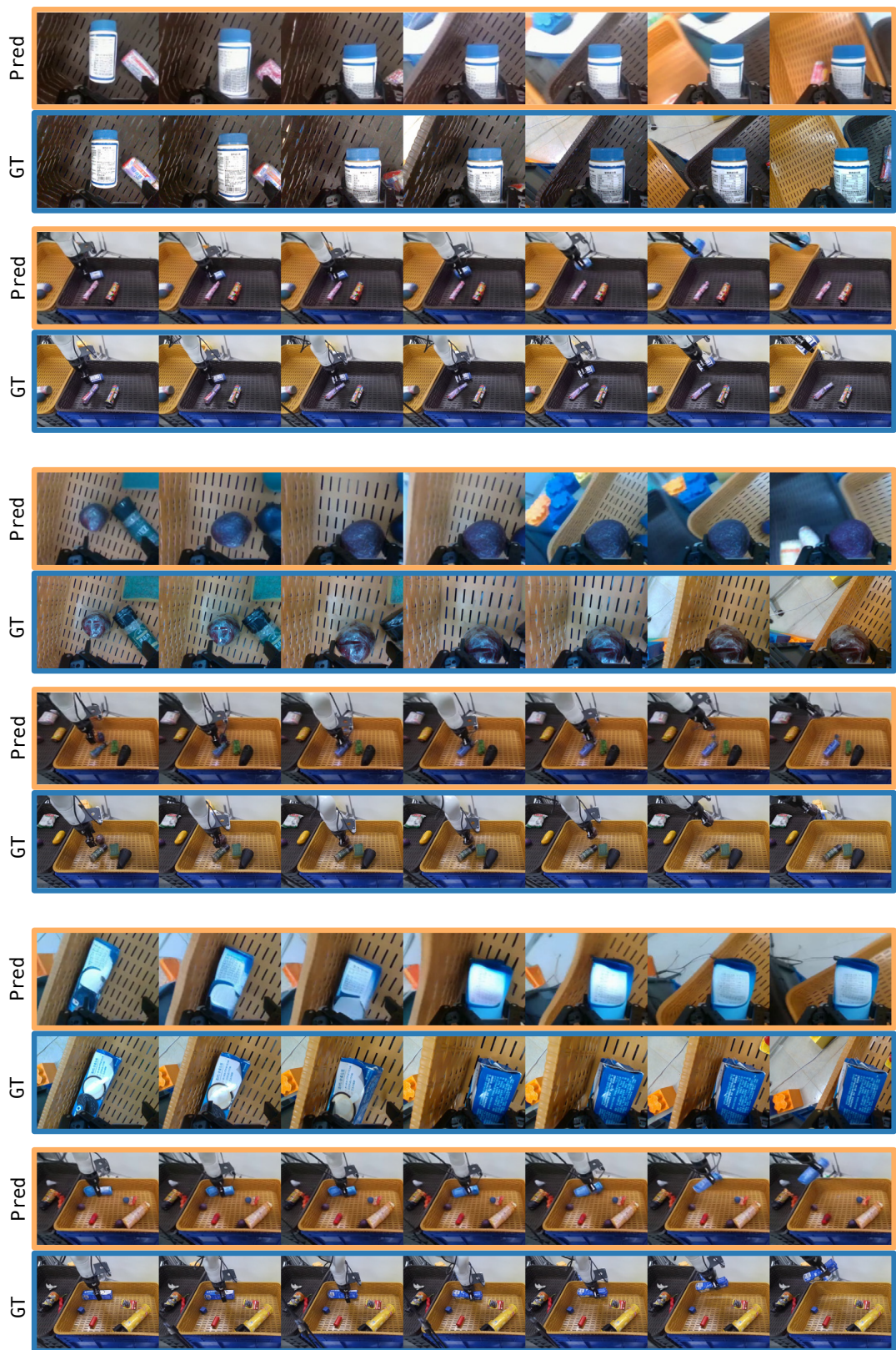
Figure 15: Video Prediction (Pred) and Ground-Truth (GT) Rollouts of End-to-End Bin Picking (II). We show autoregressive video predictions alongside the corresponding ground-truth videos captured from real-world rollouts. Both the views from the hand camera and the static head camera are shown.
