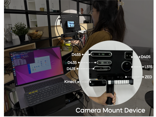
Figure 3 Multi-camera mount device for capturing the color-depth image pairs from multiple depth cameras all at once. We mount seven cameras, including five RealSense cameras (D405, D415, D435, D455, L515), a ZED camera, and an Azure Kinect camera. For the Zed camera, we record the raw data and replay it with its 4 modes (performance, ultra, quality, neural) offline. In practice, we use two computers to capture all the data due to the USB bus bandwidth limits.
