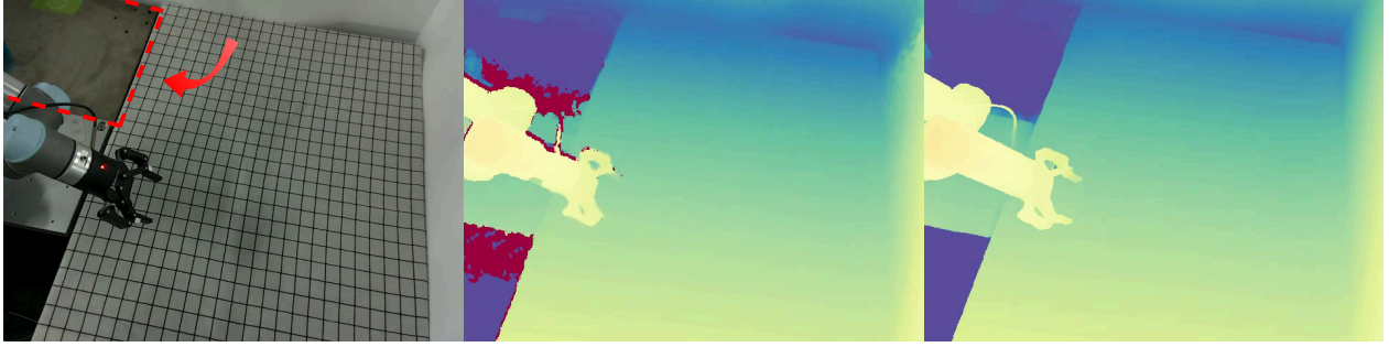
Figure 14 A typical failure case of CDM-515, caused by the wrong prompt and the less informative semantic information contained in the RGB image.
